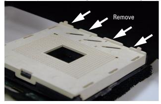
**2** Check that the socket on the target system is still open. If necessary, lift the lever of the ZIF socket on the target system.
