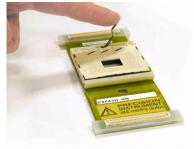
**2** Align the processor over the socket on the interposer.
