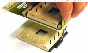
**3** Bend the flexible "wings" of the interposer upward, then align the interposer over the socket on the target system.
