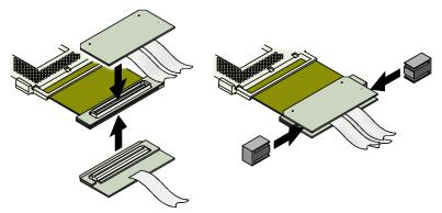
**2** Connect the analysis probe to the logic analyzer.
