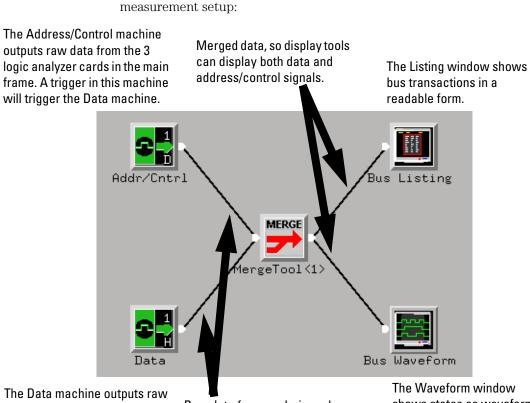
data from the 5 logic analyzer cards in the expander frame.
